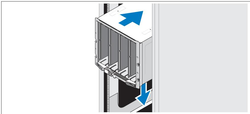
Assemble the rails and install the system in the rack following the safety instructions and the rack installation instructions provided with your enclosure.
