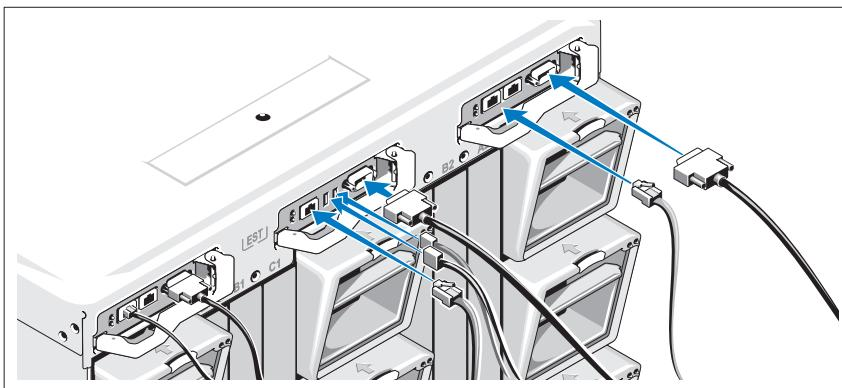
Connect the serial cable and network cable(s) from the management system to the CMC module. If a second, optional CMC module is installed, connect it as well.
